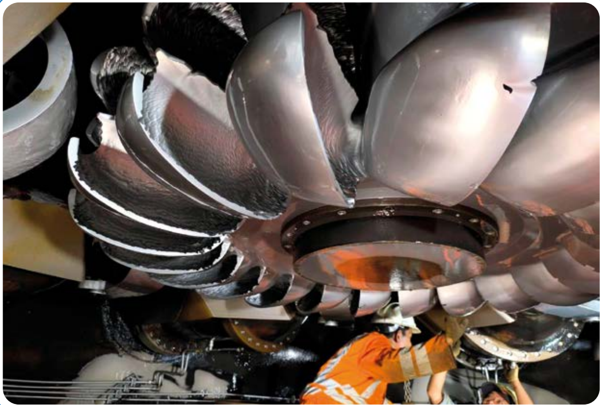
Eroded Runner of MKHEP
